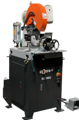
SC-350 | Solid 2.362" Tubing 4.331" Semi-Automatic Circular Cold Saw
